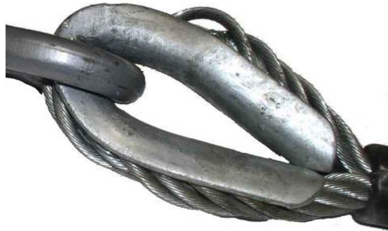
Figure 8. Deformed Thimble and Hook
