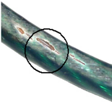
Figure 5. Damaged plastic coated wire rope.
